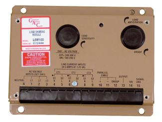
The line current measurements are usually taken from Current Transformer's (CT) existing in the equipment such as those used for ammeters. The load sharing module adds a small additional burden of only 1.25 VA to each transformer. Added cabling may also increase the burden. For example, a 0.1 ohm cable resistance is an additional 2.5 VA.
